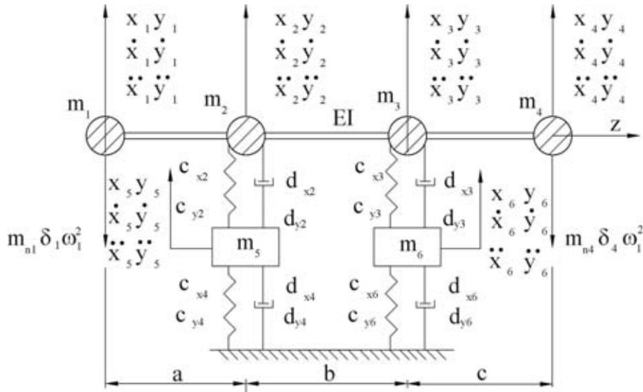
Fig.1 Model of a rotating set
