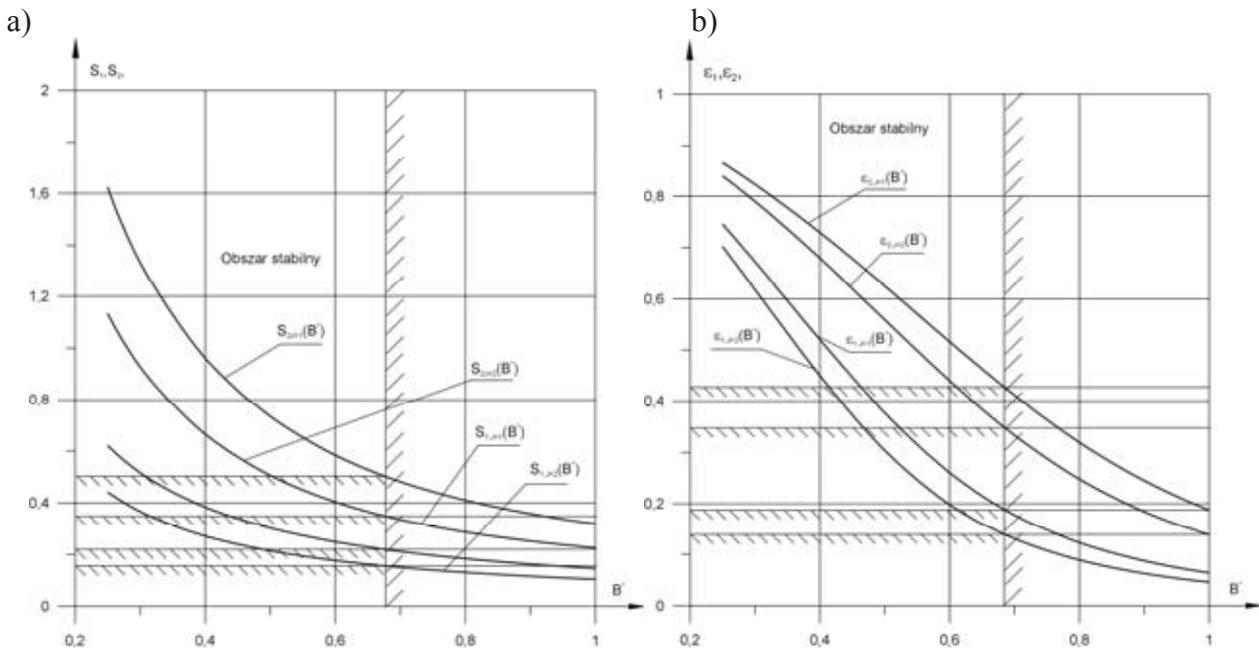
Fig.4. Stable work ranges, the influence of relative width of bearing bushes on: a) Sommerfeld Numbers, b) relative eccentricities
