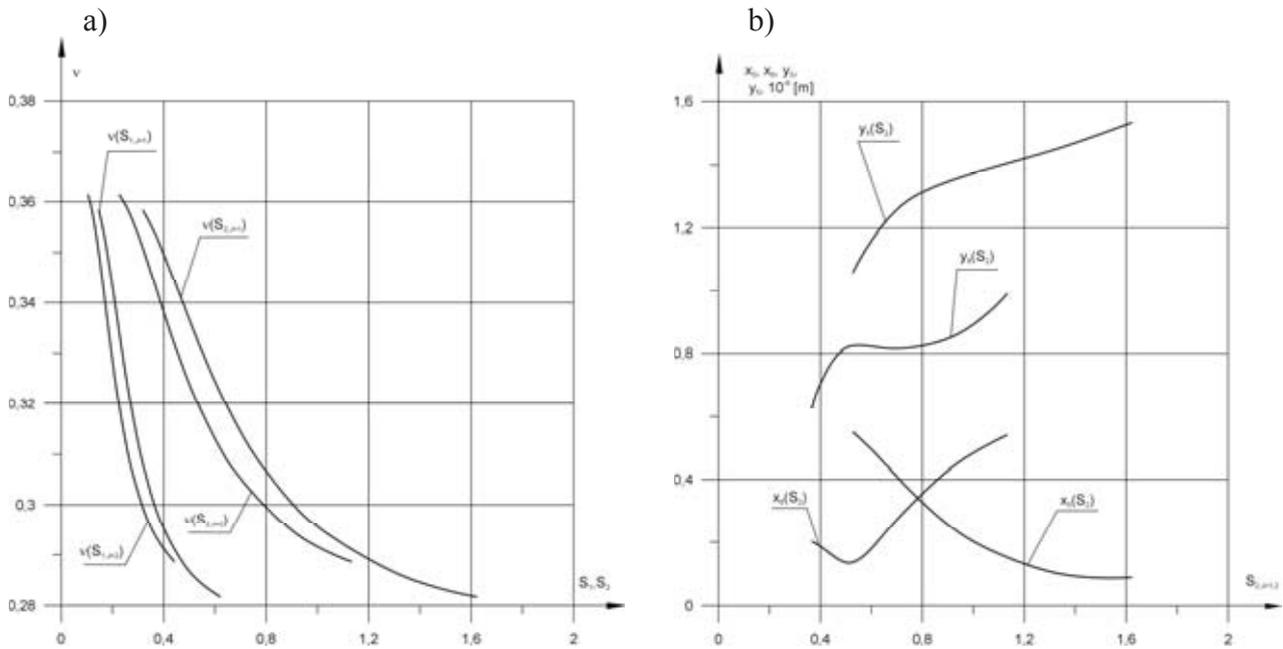
Fig. 5. a) The velocity quotient of the bearing journal and the floating ring in Sommerfeld Number function, b) The velocity quotient of the bearing journal and the floating ring in relative width of bearing bushes function
