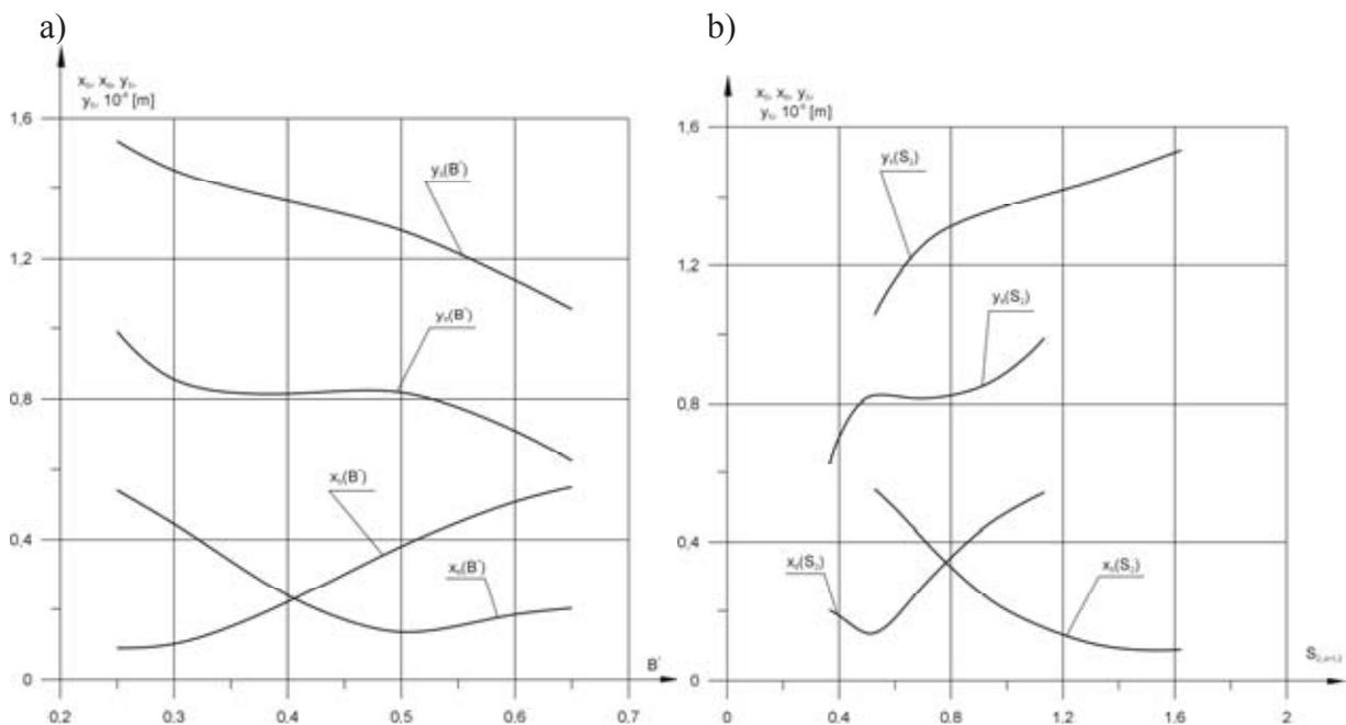
Fig. 6. a) Amplitudes of displacements in bearing knots in the function of relative width of bearing bushes, b) Amplitudes of displacements in bearing knots in Sommerfeld Numbers function
