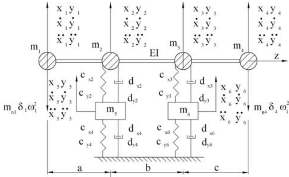
Fig.1 Model of a rotating set
