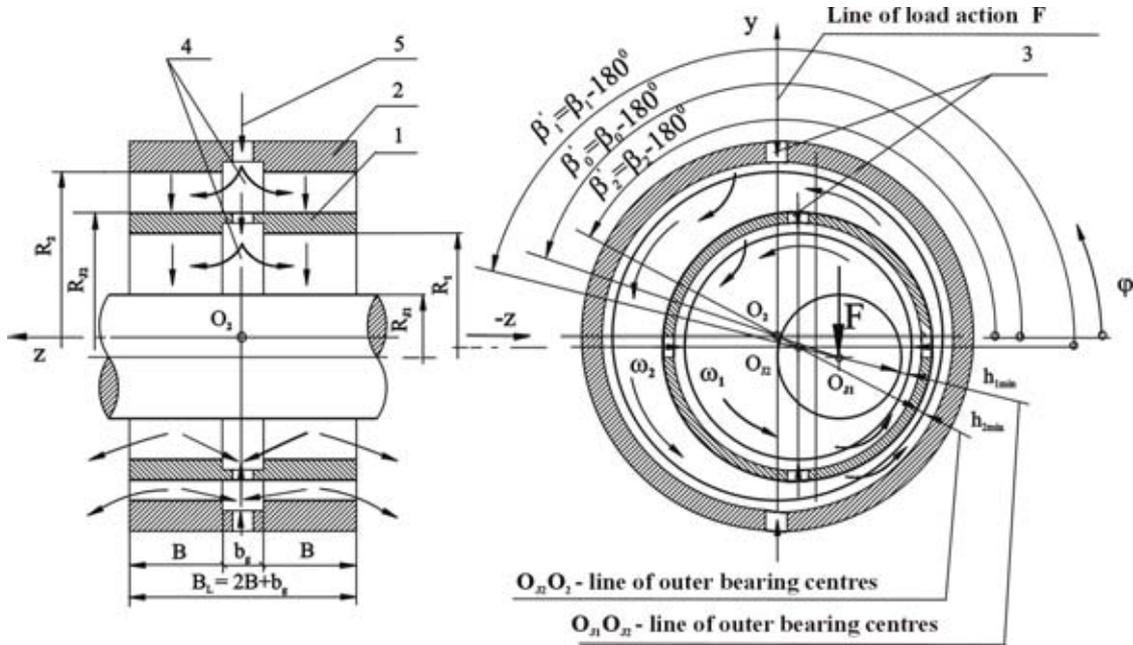
Fig.2. The sliding bearing with the floating ring: 1- the fixed bearing bush, 2- the floating ring, 3- the holes in the fixed bearing bush and the floating ring, 4- circumferential lubricant grooves in the fixed bearing bush or the floating ring, 5- directions of oil flow in a bearing
